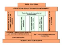
Outline of the safety concept for a KBS-3 type repository for spent nuclear fuel in a crystalline bedrock. Posiva 2012-03, Figure 5.1, P. 52.
